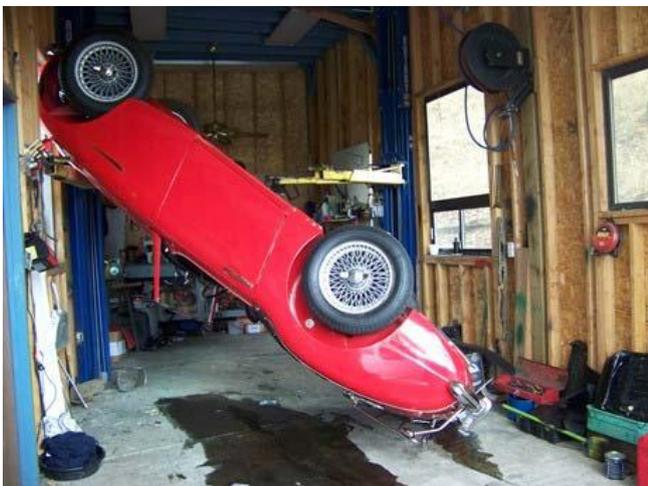
This owner failed to set the lift correctly and the car fell off. The wrecker service used a large crane to haul it out upside down and then righted the car while in the air.
