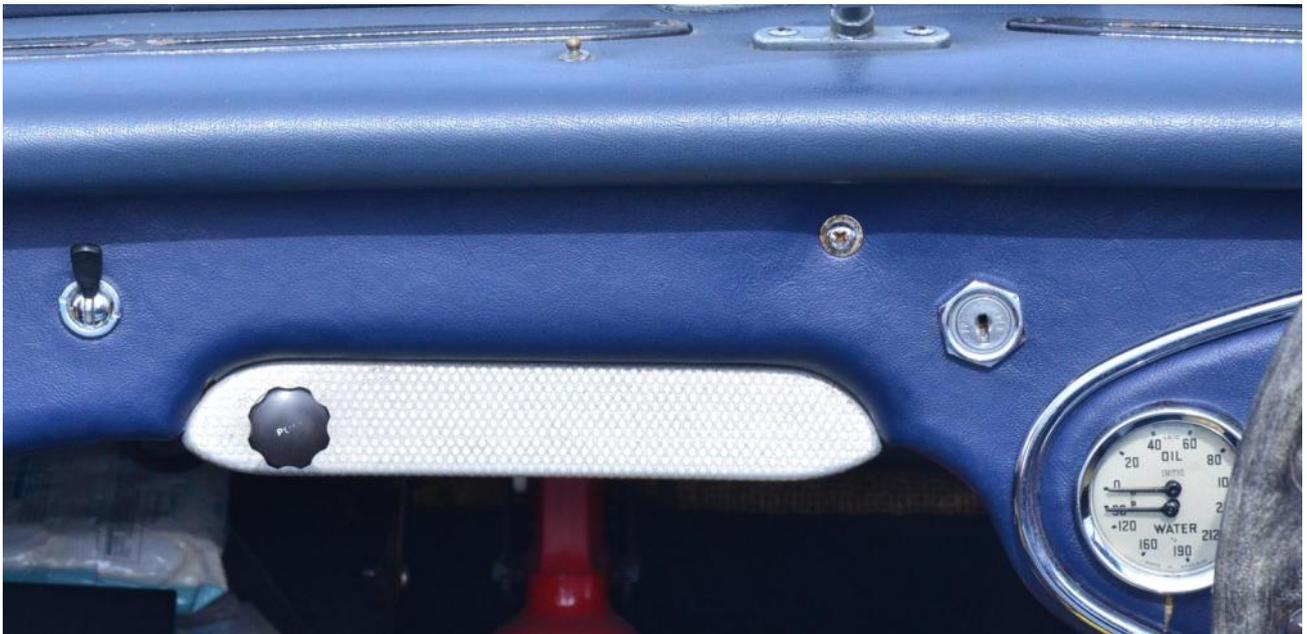
If you did not order a heater the control panel was replaced with an aluminum blanking plate similar to this one. It is made of the same material as the kick plates on the doors.
